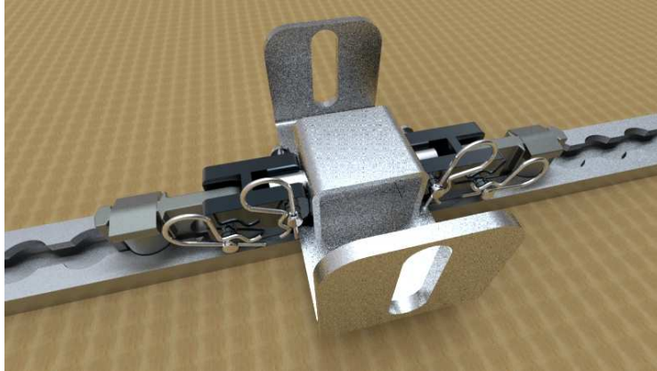
Figure 2: Swing the bracket down so that the pin-hole lines up with the opening in the A-track clip. Insert pin through bracket and A-track clip and secure into place with the hitch-clip provided
