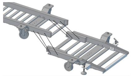
3. Attach Extension Assembly to Rear Section using (2) 3/8"x5-1/2" Bolts, (4) 3/8"x3-1/2" Bolts, (6) 3/8" Locknuts, and (12) 3/8" Washers. Be sure to insert the bolts from the inside to outside of the assembly so that they will not interfere with the wheels of a motorcycle.
