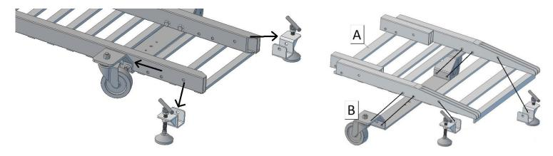
2. Attach Caster Bracket (B) and the Stop Brackets that were removed in Step1 to Extension Frame (A) using the hardware provided (C). Be sure to insert the bolts from the inside to outside of the assembly so that they will not interfere with the wheels of a motorcycle. If the fit of the wheel brackets seems too loose, use a combination of the enclosed shims (D) to fill the space on the sides of the Dolly Extension frame for a tighter fit.
