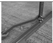
**4.** Remover High torque nut, lock washer and spacer washer from Foot Lever Arm hardware.
