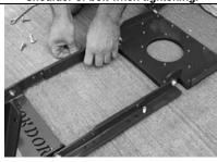
Lower the Base Plate Angle Arms onto the Top Plate Angle Arms, making sure to align the holes at the desired height setting.
